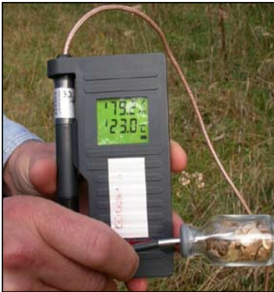
Figure 6 Checking equilibrium relative humidity of a seed sample in the field using a hygrometer. (© RBG Kew)
