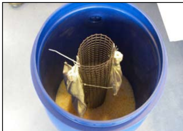
Figure 16 Drums of silica gel can be used in the field to dry seed. (© RBG Kew)
