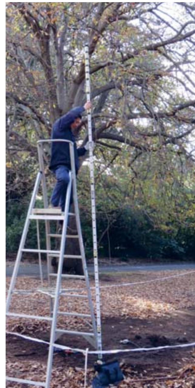
Figure 11 Four-metre deep soil moisture sensor probe on Oak Lawn 1*
